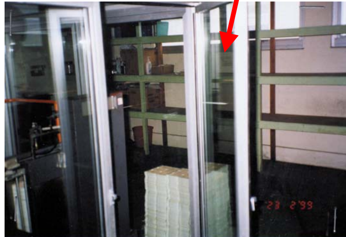
Machine enclosure mounted on damping material
