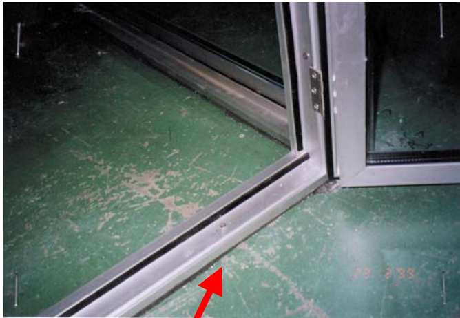
Machine enclosure mounted on damping material
