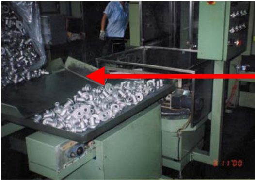
Polyurethane layer on receiving tray
