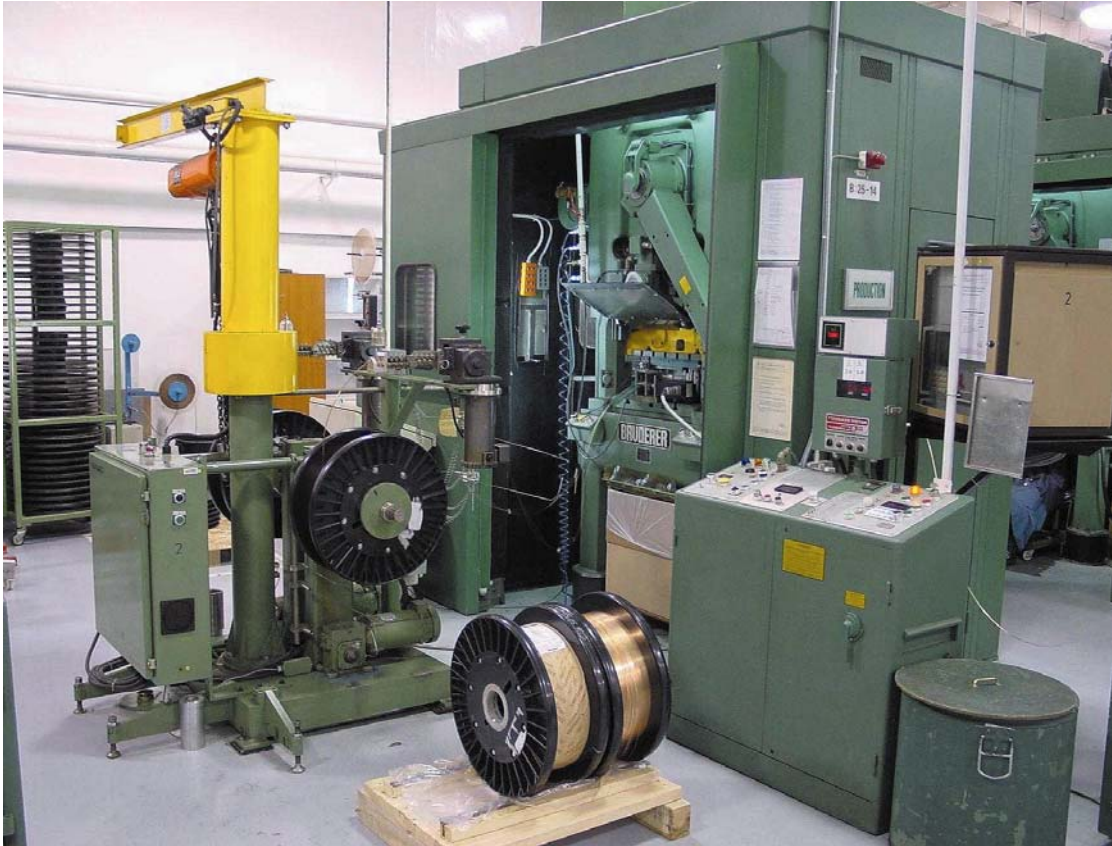
Photograph of a high-speed reel-to-reel stamping machine.
